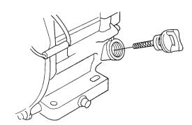
Figure 8. Engine Oil Dipstick (Removal)
